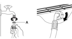
The other end of the inlet hose which connects to the machine can be turned in any direction. Simply loosen the fitting, rotate the hose and retighten the fitting, making sure there are no water leaks.
